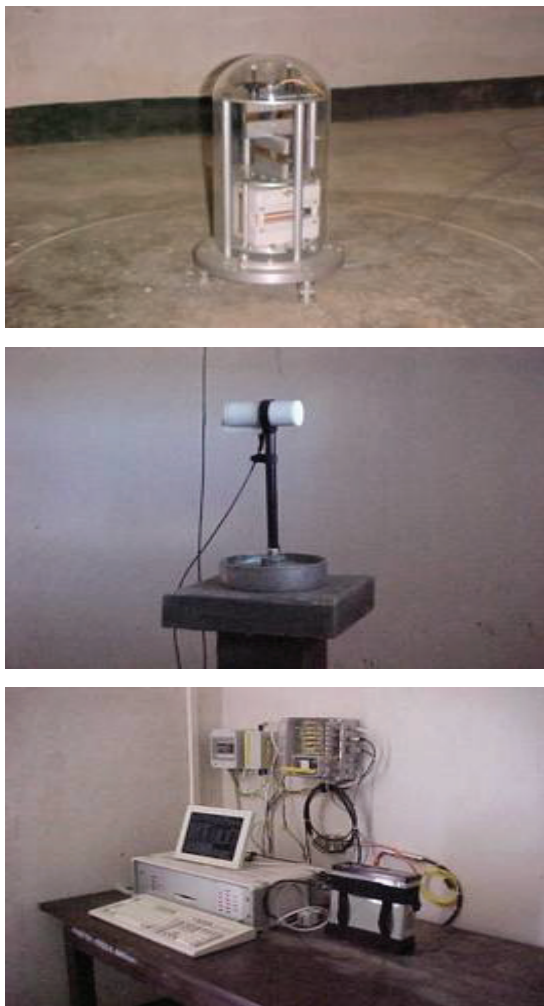
Figure 2: (Top) 3-component Fluxgate sensor head (modern variograph) installed in Villa Remedios, together with a (middle) proton precession magnetometer and (below) data-logger recorder
